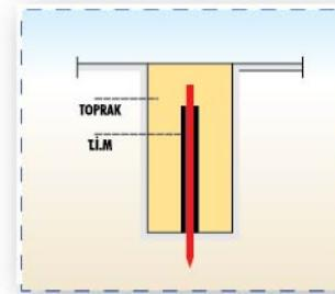
► The soil inside the hole is compressed so that the contact of SCM around the electrode and the soil intensifies.
