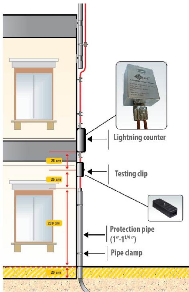
**Types of Lightning Counter:** We have three types of Lightning Counters:
