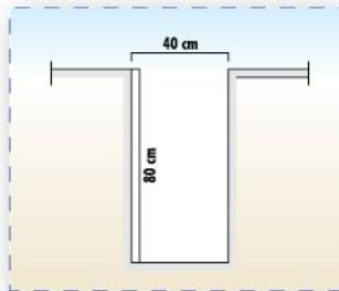
► It is necessary to dig a hole of 70-80 cm. in height and 30-40 cm. in width, where earthing electrode will be applied.
