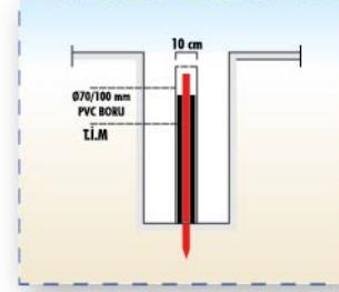
► The electrode should be placed right in the middle of the pipe and then the pipe should be filled with SCM, leaving the upper 10 cm part of the electrode open.
