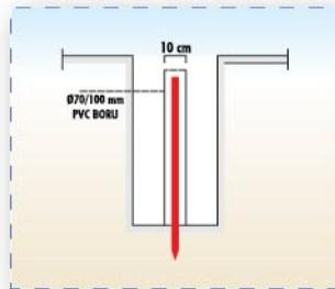
► The electrode is nailed 10 cm. below the surface and the rod should be covered by a PVC pipe with a diameter of 70 to 100 mm.
