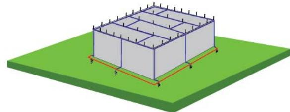
In practice, the roof and sidewalls of the building are covered with good conductive material vertically and horizontally, thus taken in a cage. Vertical pointed rods are placed on the roof at regular intervals and are connected to the cage. The cage is then connected to the earth at many points with the use of conductors and grounding electrodes on the base.
