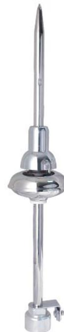
(\*)  $\Delta t$  value shows the early streamer time advantage that a lightning rod (ESE lightning rod, for instance) has in arresting the lightning, compared to an ordinary capture terminal (S.R.). Bigger  $\Delta t$  value means that the active reaction of the lightning rod is better. It shows that it can attract the lightning to itself at a higher point, at a larger protection diameter and fastly. )
