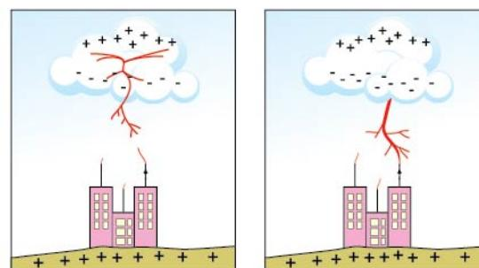
The lightning discharge occurs not with jumps, but with the passing of a strong current through just one conductive path, which may be followed by second or third discharges. The lightning is not an ultrasonic incident, but a unipolar shocking discharge; a short wended, direct current stroke, measured to be of 20-100 million volt with 5-200 current value.
