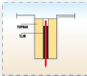
► The area outside the PVC pipe (electrode hole) is filled and closed by soil.
