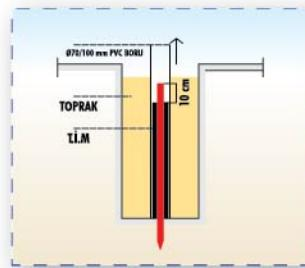
► The PVC pipe surrounding the electrode is pulled up and displaced.
