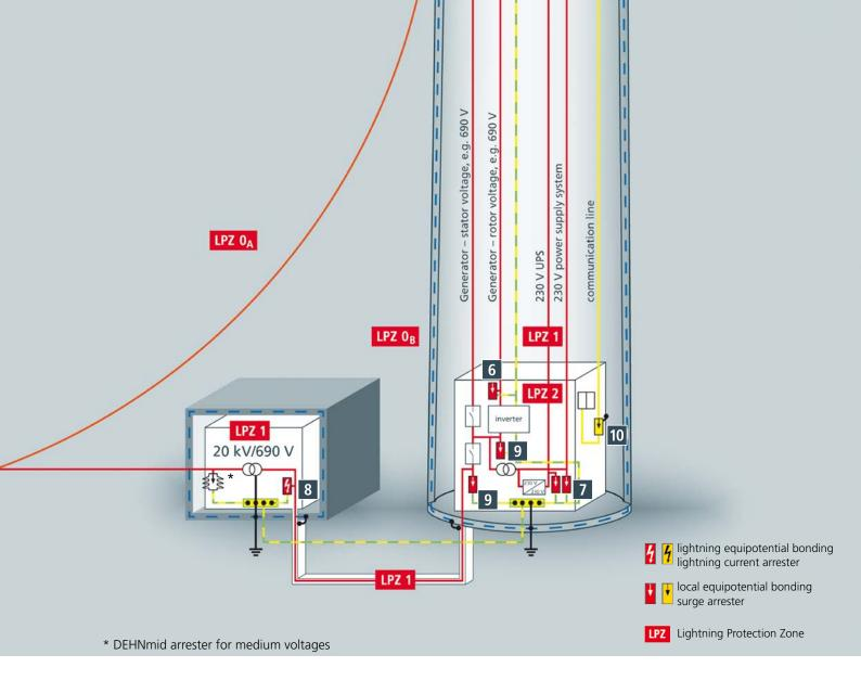
The IEC 61400-24 standard recommends to dimension the lightning protection system of a wind turbine according to class LPS I unless a risk assessment demonstrates that a lower LPS class is sufficient for the individual components.
