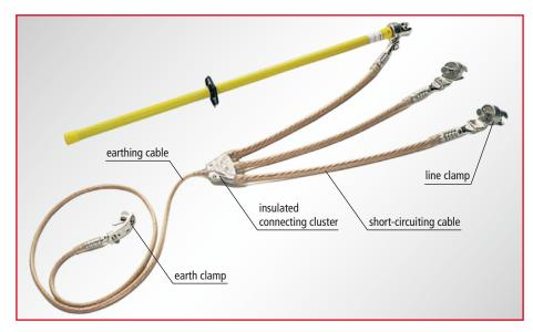
Earthing and short-circuiting device in accordance with EN 61230, new equipment with ball head cap and earthing rod
