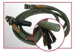
Faulty earthing and short-circuiting device, short-circuiting cable with advanced black colouration
