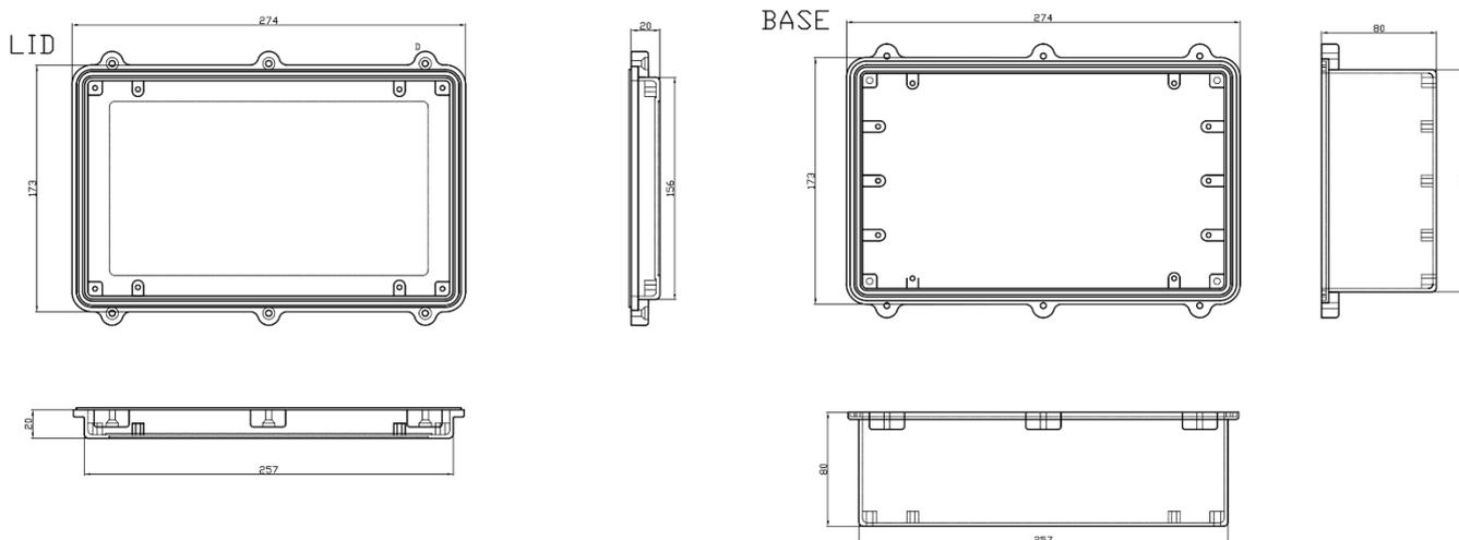
IP67 base complete with gasket, aluminium light grey painted, surface mount via external feet
